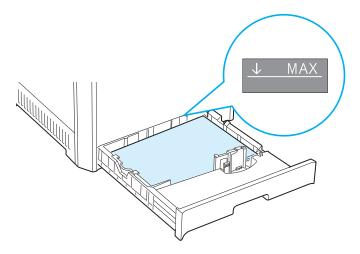
6 Pinch the paper guide as shown and move it towards the paper until it lightly touches the side of the stack. Do not press the guide too tightly against the edge of the paper as the guide may bend the paper.
